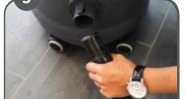
Apply vacuum lid and connect the hose to the machine.
